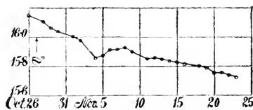
FIG. 23.—Chart showing loss of standard volumes of gas in diver in lapse of days. Diffusion of air through KCl solution.
